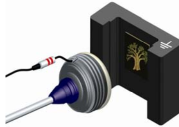
The vacuum is released at the same time as the static is turned on passing through the foam pad, charging the label and pinning it to the tool.
